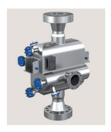
**PCHE**s are constructed from flat metal plates into which fluid flow channels are chemically milled. The chemical milling technique is similar to that employed for manufacturing electronic printed circuits. This method of manufacture gave rise to the name 'Printed Circuit Heat Exchanger'.
