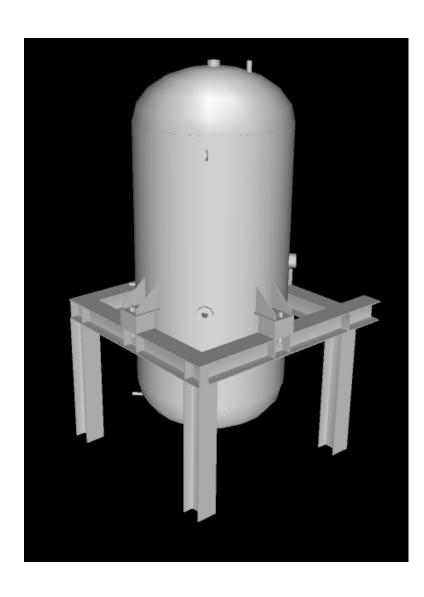
**SEPARATOR** fluids enter the vessel through an inlet device whose primary objectives are to achieve efficient bulk separation of liquid from he gas and to improve flow distribution of both phases through the separator.
