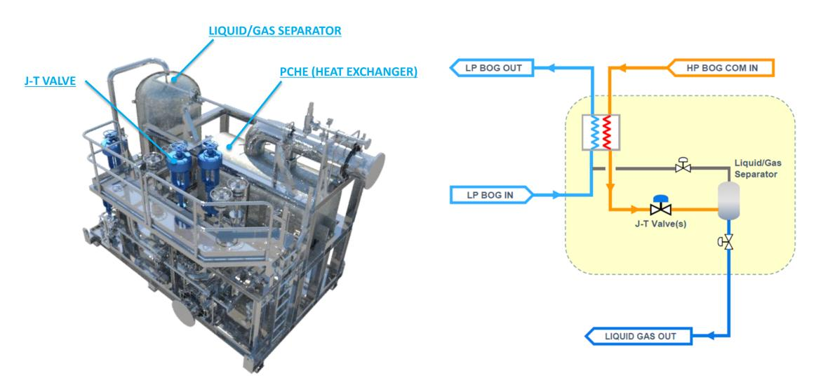
Separation efficiency (BOG → liquid) : less than 70% (based on NBOG)
