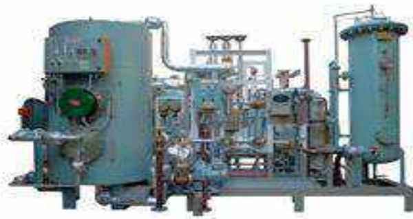
Fresh Water Generator Unit
