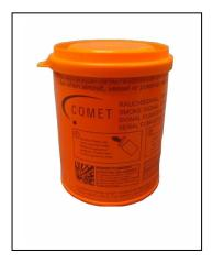
**Smoke Signal:** Approved according to EC. Distress signal for lifeboats and liferafts that conforms to SOLAS 74/88. Floating smoke buoy for marking purposes. The smoke signal, is equipped with a pull-wire igniter. The smoke duration is 3 minutes.
