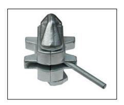
**Left Locking Twistlocks:** Housing – Ductile Iron, Cone – Drop Forged & Finish – Hot Deep Galvanised. Min Break Load – 40 Ton
