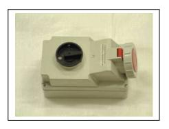
Mennekes Switched Socket with Interlock: Interlock mechanism prohibits the switch from being turned "ON" unless the plug is fully inserted. The plug cannot be removed unless the switch is in the "OFF" position.
