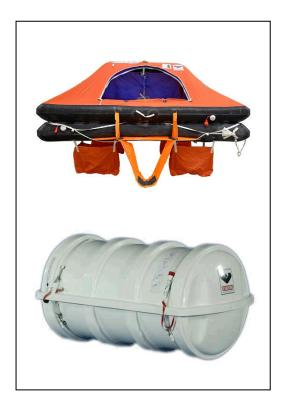
Life raft Throw Overboard: Type DK+. Approved according to SOLAS LSA-code, EC directive 96/98/EC and USCG. Throw overboard life raft. The throw overboard life raft is released from its cradle and thrown overboard, or slides automatically when released. Once waterborne, the life raft inflates on a hard pull of the painter line and is then ready for boarding. Delivered in a square or round fibre-glass container. Available in 4, 6, 8, 10, 12, 16, 20, 25 or 35 Persons
