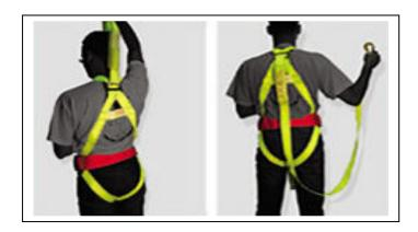
**Full Body Harness**: For working at height. Full Shock Absorption. Heavy duty webbing. SABS - EN 358:1992. SABS - EN 354/355:1992. Do not remove sleeve from shock absorption lanyard. Replace if used in fall arrest situation. Safety blocks available.
