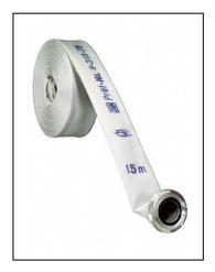
**Fire Hose Standard:** Width: 1.5", 2" or 2.5". Coupling: Storz C, Storz 38 or Storz 65. Material: Aluminium or Brass. Colour: White. Length: 10, 15, 20 or 25 metre. Other Couplings or Lengths available on request.
