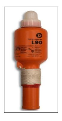
**Lifebuoy Light:** Approved according to EC. Lifebuoy marker conforming to SOLAS 74/88. The lifebuoy light is a dry cell powered light equipped with a tilt switch for automatic function. It burns for two hours with a light intensity of at least 2 candela and is safe on oil- or petrol covered waters.
