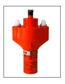
Light-Smoke Signal (MOB): with Lithium Battery. SOLAS. Approved according to EC. Equipment for marking a lifebuoy in manoverboard situations. The smoke signal will be activated by a pull wire igniter and the electric lights will be switched on by a tilt switch. The smoke signal emits dense orange smoke for a total of 15 minutes. The signal is safe on oil or petrol covered water. The signal is manufactured of seawater resistant aluminium and plastic
