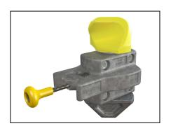
**Semi-Automatic Twistlocks:** Housing – Ductile Iron, Cone – Drop Forged & Finish – Hot Deep Galvanised. Min Break Load – 50 Ton
