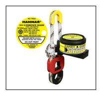
Hydrostatic Release Unit for Liferafts: with Shackle. Hammar H20. Approved according to USCG and EC. The Hammar H20 is a hydrostatic release unit for all types of liferafts. It is made of glass fibre and reinforced nylon that enables liferafts to surface and inflate when a ship is sinking.
