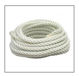
**Nylon Rope:** 3 Strand. General purpose rope for dynamic loading. Nylon has excellent stretch and recovery characteristics, and is used in many anchoring and mooring applications. When new, nylon ropes can stretch up to 35% of their length before break. Stretch characteristics will reduce relative to the amount of use and can lose 10% of its tensile strength when wet.
