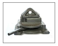
Bottom Twistlocks – 45/55 degrees: Housing – Ductile Iron, Cone – Drop Forged & Finish – Hot Deep Galvanised. Min Break Load – 30 Ton
