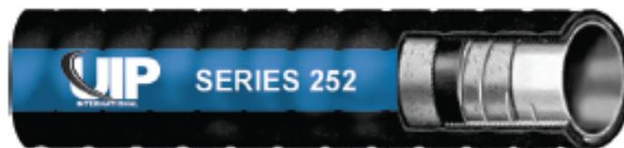
Compounded to resist engine heat, exhaust fumes, ozone, mild acids, toilet effluent, saltwater, and abrasion. Meets or exceeds USCG, ABYC, and SAE J2006 R2 Standards for wet exhaust service. Designed for severe-bend applications.
