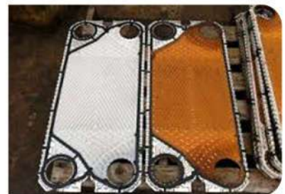
HEAT EXCHANGER PLATE BEFORE & AFTER CHEMICAL CLEANING
