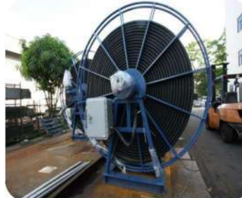
Hose Reel System
