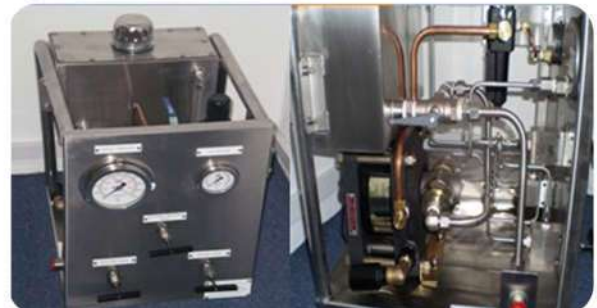
PRESSURE TESTING PUMP
