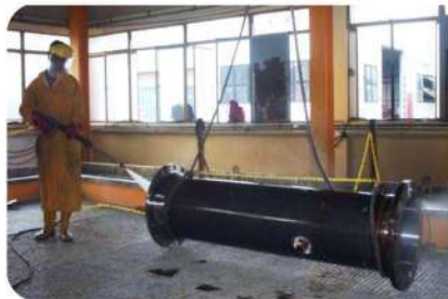
HIGH PRESSURE WASH
