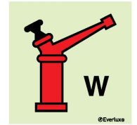
S 10 38 Water monitor (gun)
