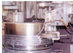
Grinding of piston crown
