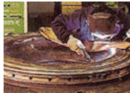
TIG Welding of cylinder cover
