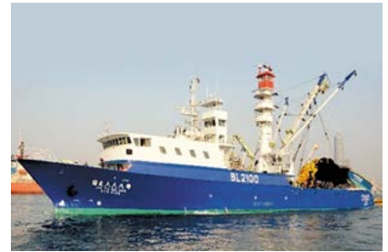
Ri You 668, offshore purse seiner, Ri You Fishery Corporation 8DKM-28e × 1, Zhong Xin Shipbuilding Corporation
