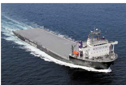
Yamatai, heavy cargo ship, NYK Bulk & Projects Carriers Ltd. 6DKM-36e(L) × 2, Nagasaki Shipyard & Machinery Works, Mitsubishi Heavy Industries, Ltd.
