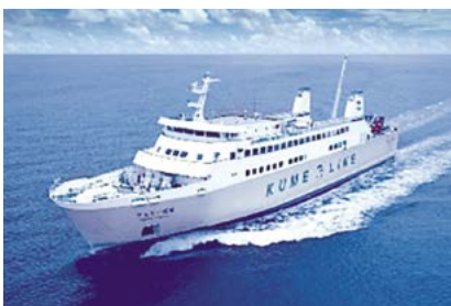
Ferry Ryukyu, ferry, Kume-Shousen Co., Ltd. 8DKM-28e(L) × 2, Usuki Shipbuilding Co., Ltd.
