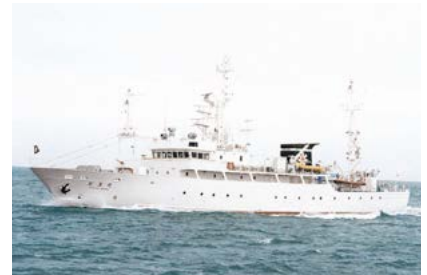
Hokuo Maru, fishery control boat, Hokkaido Government 6DKM-28(L) × 2, Narasaki Shipbuilding Co., Ltd.
