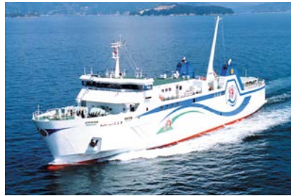
New Koshiki, ferry, Koshikishima Shosen Co., Ltd. 6DKM-28(L) × 2, Kanda Shipbuilding Co., Ltd.
