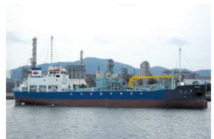
Tokuyama Maru, cement tanker, Tokuyama Kairiku Unso K.K. 6DEM-23F × 1, Yamanaka Shipbuilding Co., Ltd.
