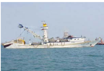
Feng Guo 869, purse seiner, Feng Guo Fishery Corporation 8DKM-28e × 1, Qing Fu Shipbuilding Corporation
