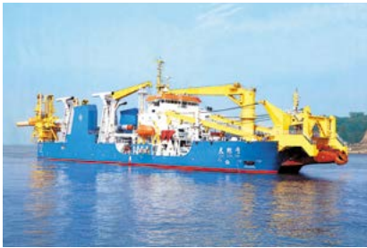
Tianjing Hao, 4,500 m3 self-propelling dredger, Tianjing Waterway Bureau 8DKM-36(L) × 2, pump-driving 8DK-36 × 2
