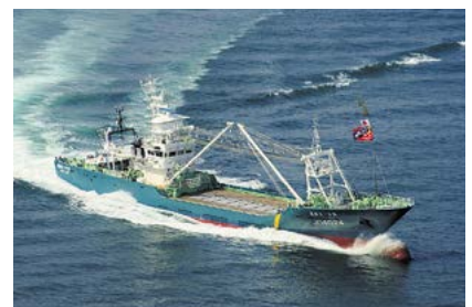
Daishimaru #11, seine accessory carrier, Daishimaru Fishery Co., Ltd., Nagashima Ltd. 8DCM-32eL × 1, Izutsu Shipyard Co., Ltd.
