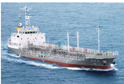
Kosei Maru, chemical tanker, Tabuchi Kaiun K.K. 6DKM-28L × 1, Maehata Shipbuilding Co., Ltd.
