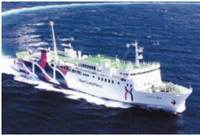
Saipia Soya, ferry, Heart Land Ferry Co., Ltd. 8DKM-28(L) × 2, Naikai Zosen Corporation
