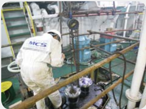
Relocate the MGPS anode from sea chest to strainer
