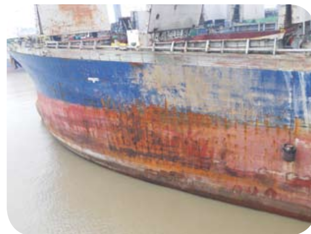
Hull conditions with defective ICCP system
