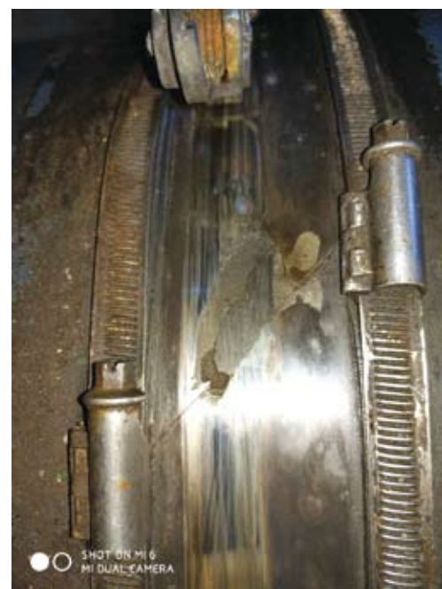
Slip ring in poor conditions
