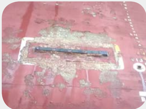
Di-electric shield in poor conditions
