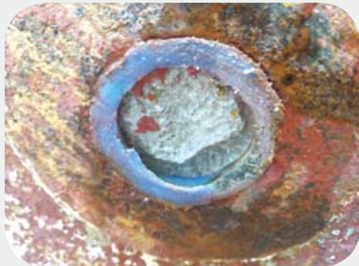
Ref. cell in poor condition
