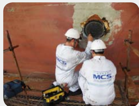
ICCP anode inspection
