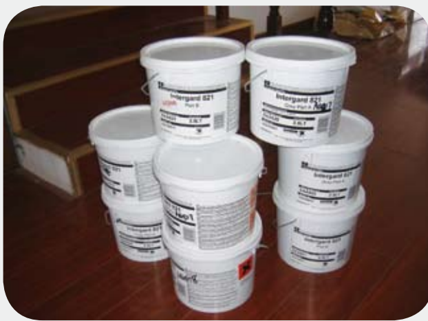
Epoxy filler for ICCP Di-electric shield
