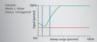
The CleverLevel LFFS switch is the solution: Thanks to its frequency sweep technology and its ability to analyze the strength of the signal, and the signal dumping which differs from media to media. The switch can be set to trigger only on the specific medium even if both media involved have the same Dk value.
