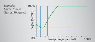
Sometimes two media might have the same Dk value. So how can they be distinguished? Setting each of the two independent switching points doesn't help here (two blue lines).
