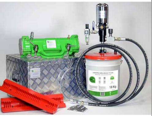
provides fast and effective lubrication of wire ropes at speeds up to 2,000m per hour. 3 VIPER kits are available covering following dimension ranges: 6-36mm (Mini), 8-67mm (Mid) and 50-165mm (Maxi). Whilst at the same time achieving more thorough results by forcing quality lubricant under high pressure right through to the core of the wire rope.
