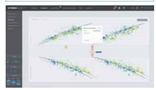
Analyzes hull condition based on ISO15016 or machine learning, and displays the trend of hull fouling and performance reduction.
