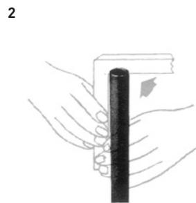
The tube is cut at a right angle.
