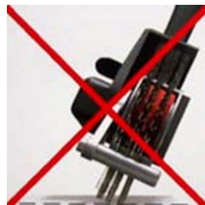
Work perpendicular to the surface
