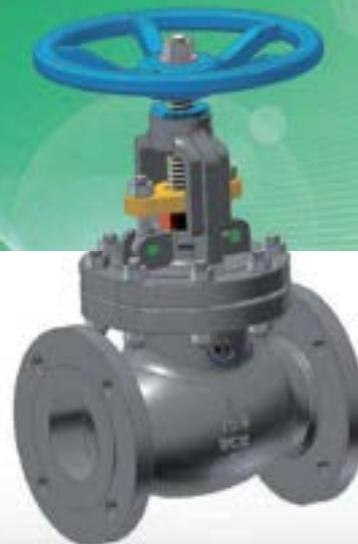
All globe valves utilize the “port closure” concept of valves. By this it meant that fluid passes through a specific opening (rather than a general passageway, as in the case of gate valves), and the fluid is controlled by means of a stem-mounted disc or inserted plug in that area.
