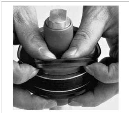
Fig. 26 Snap-in fitting of a piston seal
