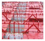
SMS-SME also provides reefer container M&R (Maintenance & Repair) platforms separately or combined with lashing bridge. Reefer containers on higher tiers can be easily monitored and repaired from the platform just in front of reefer container unit.
