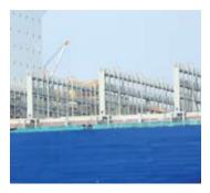
Lashing bridges are installed on container ships and designed to restrain racking forces from container stack loads and create safe spaces for reefer container monitoring, maintenance and repair.
