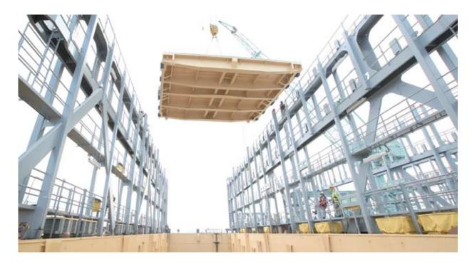
Pontoon type Hatch covers are available as single or multi panel units with non-sequential operation by using flap sealing system.
