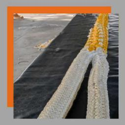
Cover in the eyes: a basic protection can be placed only on the eyes to protect them against chafing on bollards and bitts.
