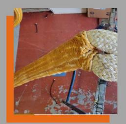
Cover in the eyes and on the leg: in addition to the jacket on the eyes a further protection can be placed on the initial part of the leg. This ensures that the most stressed areas are always protected.
