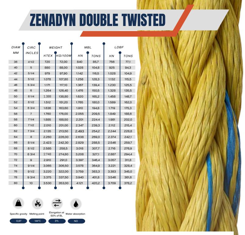
Our ZenaDyn Double Twisted has been specifically studied for towing applications to offer an unjacketed rope with superior efficiency.
