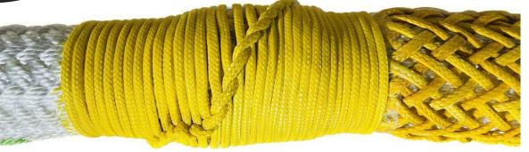
On the other side the D-Web is fixed by means of some tuck splice and all the area is then covered with a tight lashing made with a small rope, in order to reduce the volume and the risk of snagging.
