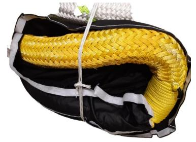
The ending yarns of the PES cover on the eyes are buried inside the core of the cable to prevent it from moving and becoming loose. This also ensure that the core is always protected and never exposed.
