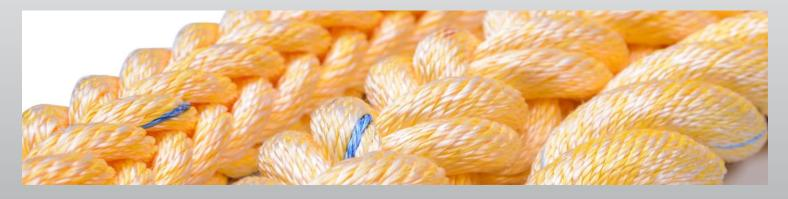
The yarns of the two fibres are twisted and then combined in different percentages to obtain the two main versions of the product, floating (with a mix of 30% PES and 70% Polyolefins) and non-floating/sinking (50% - 50%).
