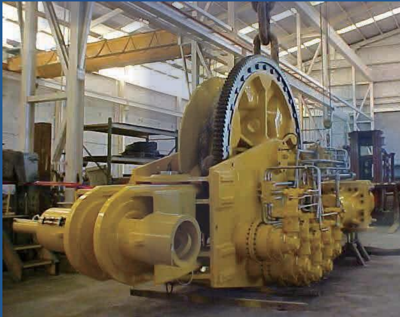
750T Chain Jack with Integral 250T Windlass
