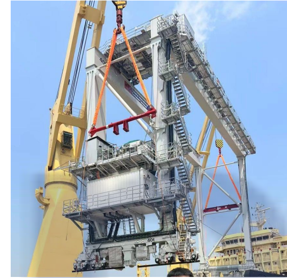
Rubber Tyre Gantry Crane (RTG) Capacity: SWL 15T - 80T
