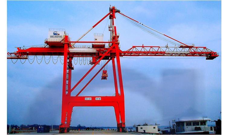
Ship-to-Shore Crane (STS) Capacity: SWL 40T - 80T
