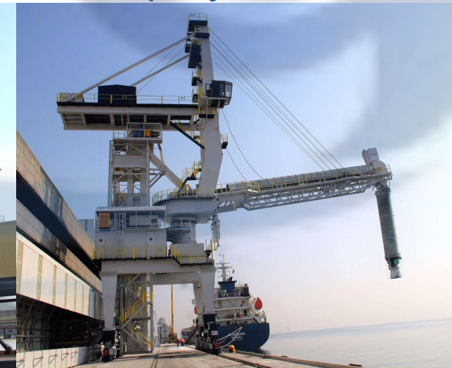
Ship Loader / Unloader Capacity: 500T/h - 3000T/h
