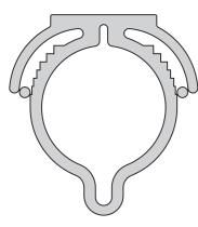
Cargo Care Solutions has developed a rubber sealing which can be pressed in the cross joint to give extra security for the weather tightness of your hatch covers. We provide 2 sizes, one size works between gaps of 20 – 50 mm and the second size works between gaps of 45 – 80mm. A complete set for 1 cross joint consists of 1 straight length of packing (cut-to-size) and 2 pieces 90Ż corners.
