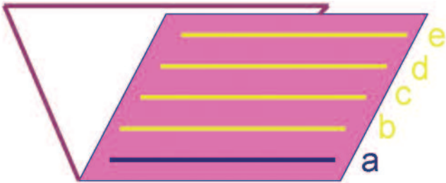
Bottom staff is transmitter, multiple receive elements.
