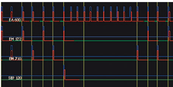
K-Sync graphic display showing systems' sequencing.
