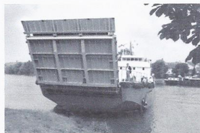
Landing vessel with hydraulic driven bow ramp
