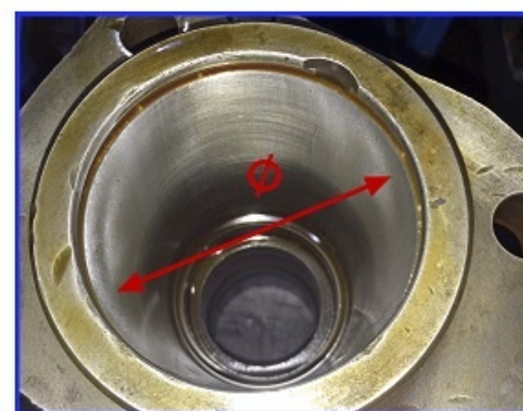
Rebuilt housing inner bore
