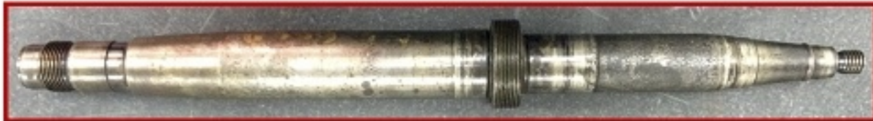
Oil purifier shaft with worn taper
