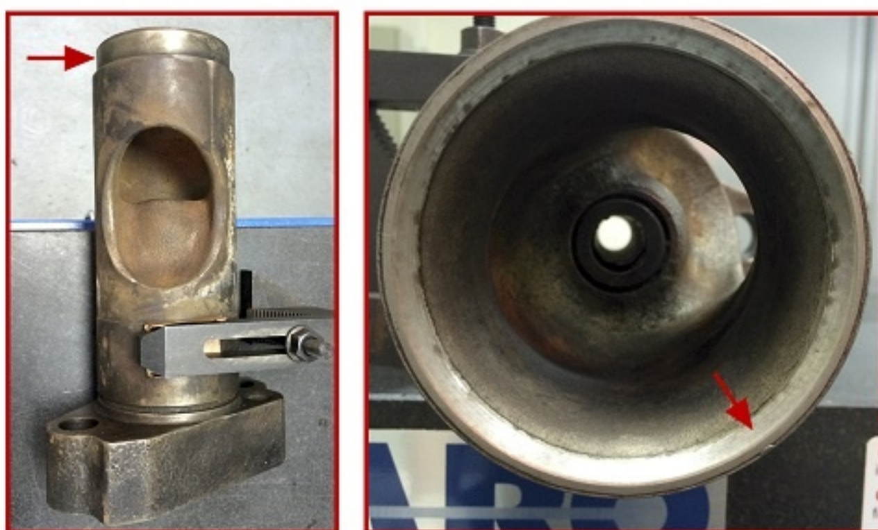
Valve cage with worn seating area
