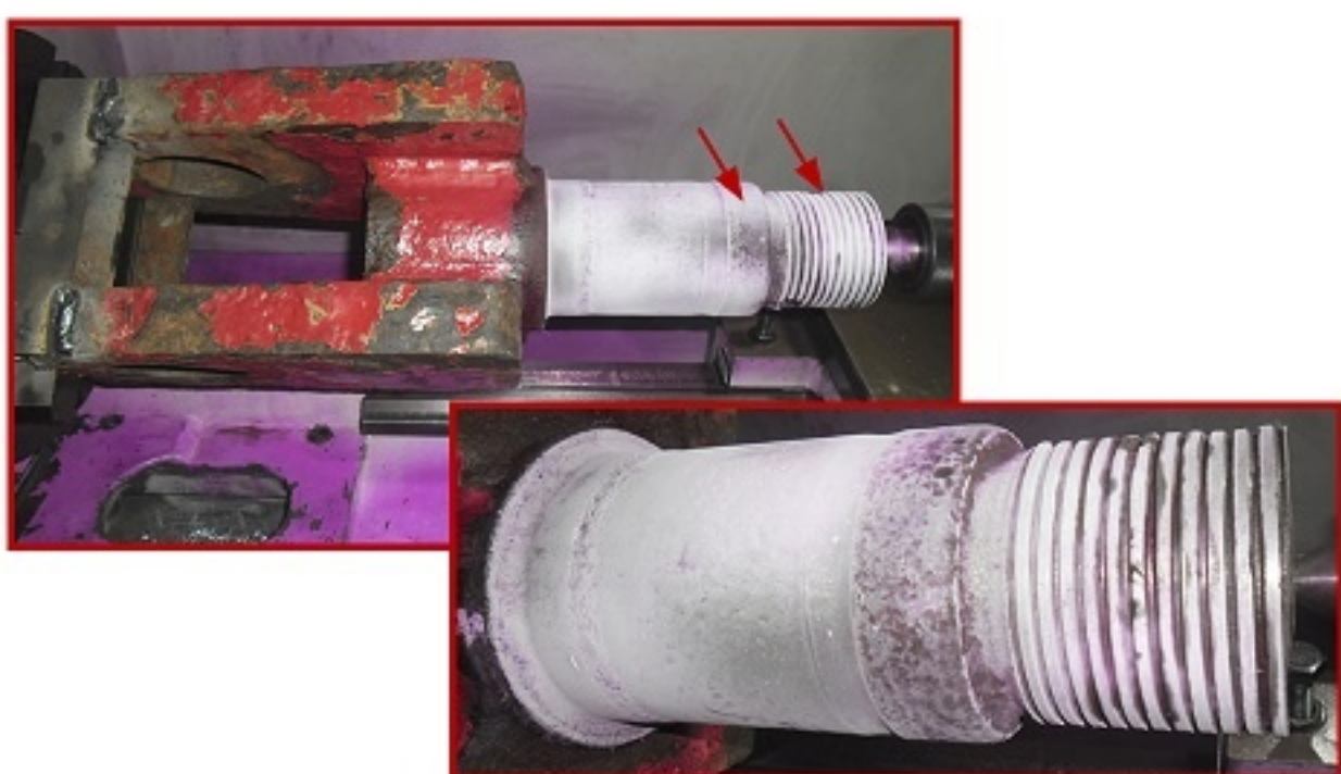
Crane Swivel shaft with damaged thread and shank
