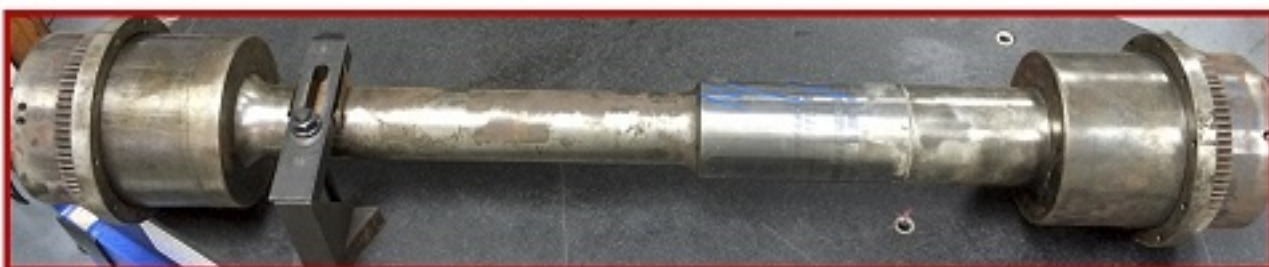
Intermediate compressor shaft with damage to bearing journal
