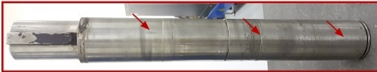
Pump shaft scoring and pitting along shaft length
