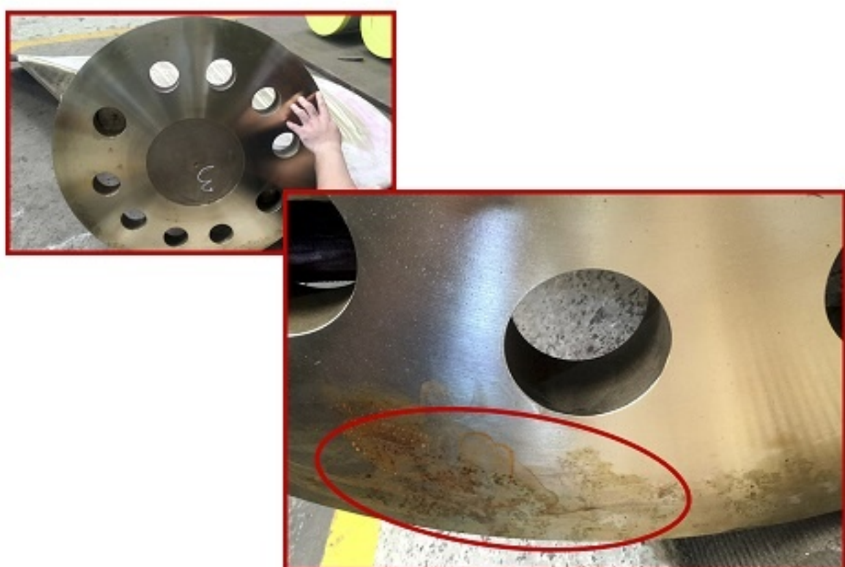
CPP blade foot landing porosity
