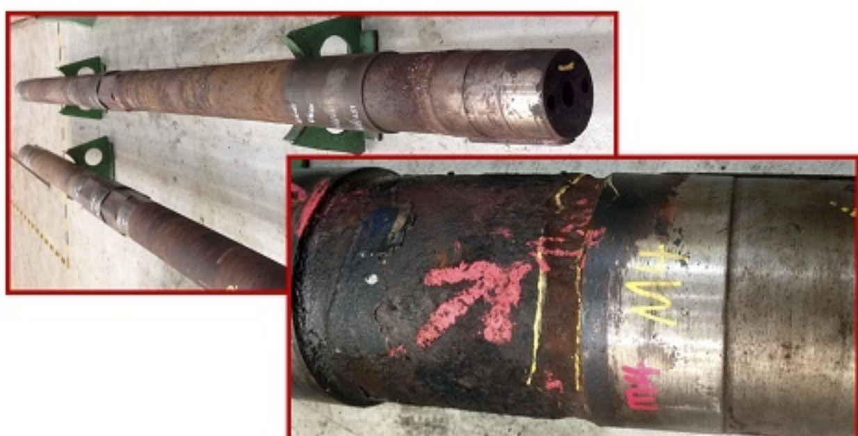
Mooring winch shaft journal wear
