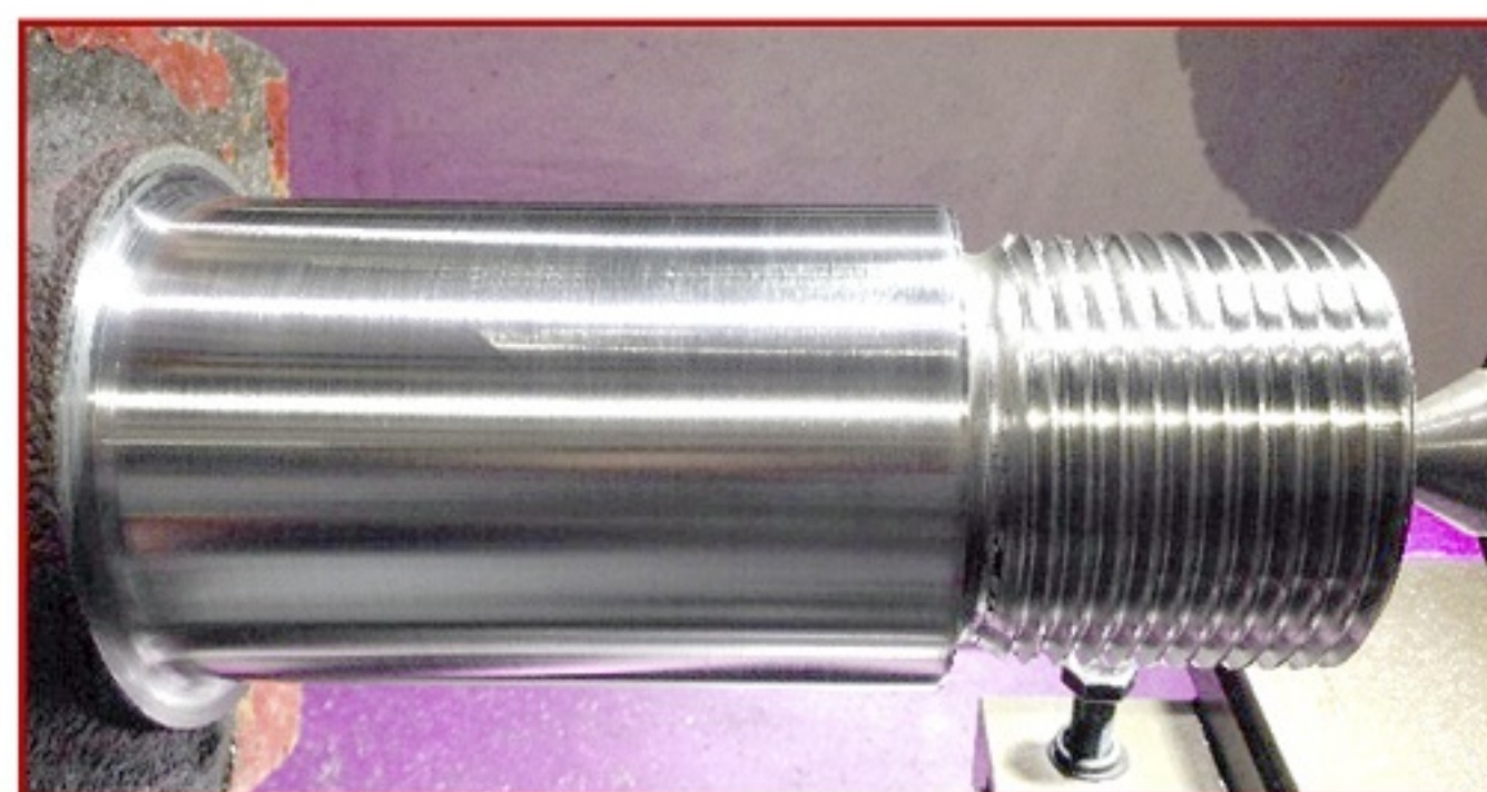
Completely rebuilt shank and thread
