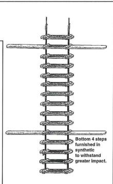
Both ladders have the A.L. DON Co. patented clamp that was designed for quick step replacement with no special tools.
