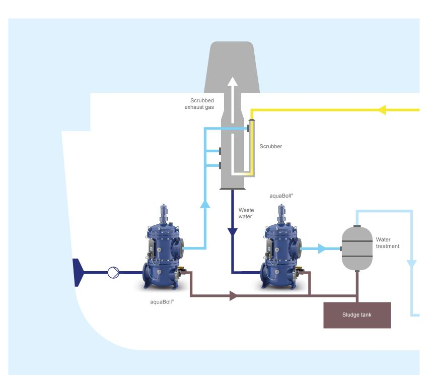
fresh water, is generated by adding sodium hydroxide (i.e. caustic soda). In both cases, permanent nozzle protection is required to continue the exhaust gas cleaning process. To this end, aquaBoll® efficiently removes organic and inorganic particles from the input medium while also ensuring fully automated filtration of the waste water generated during this process.
