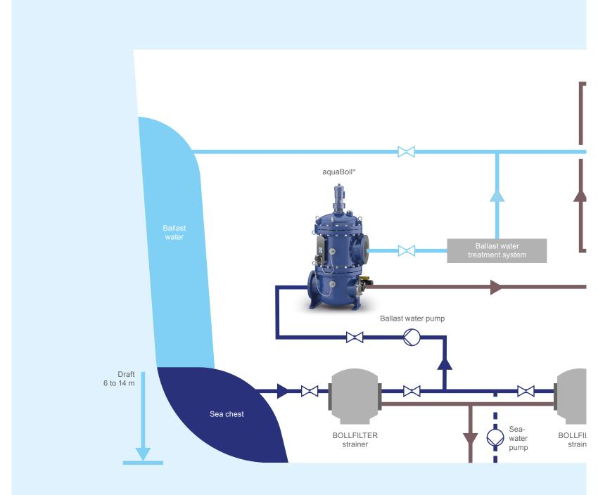
efficiency. Thanks to its innovative design and optimised functionality, the aquaBoll® guarantees the necessary filtration quality even at the highest of flow rates. The compact automatic filters are
