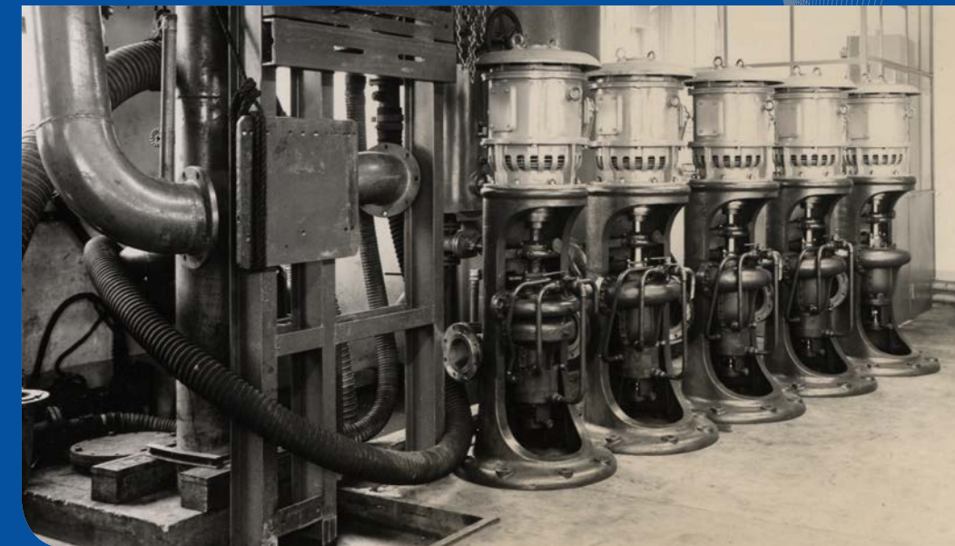
1958: Pumps for a general cargo ship on the testbed
