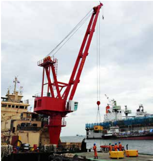
Dieseldriven Offshore Crane with wire luffing Bespoke Design
