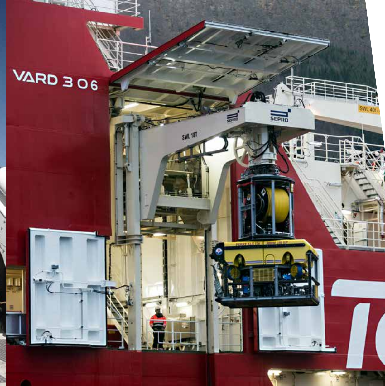
Overhead Rail System ORS™ - Gantry type of LARS with extensive lowering capabilities along the ship-side rails making launch of ROV possible below splash zone.
