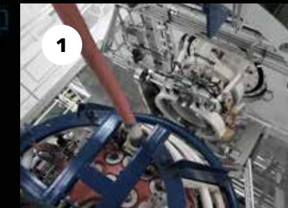
1. Passive Cursor Frame and Telescopic trunk to diver's quarters
