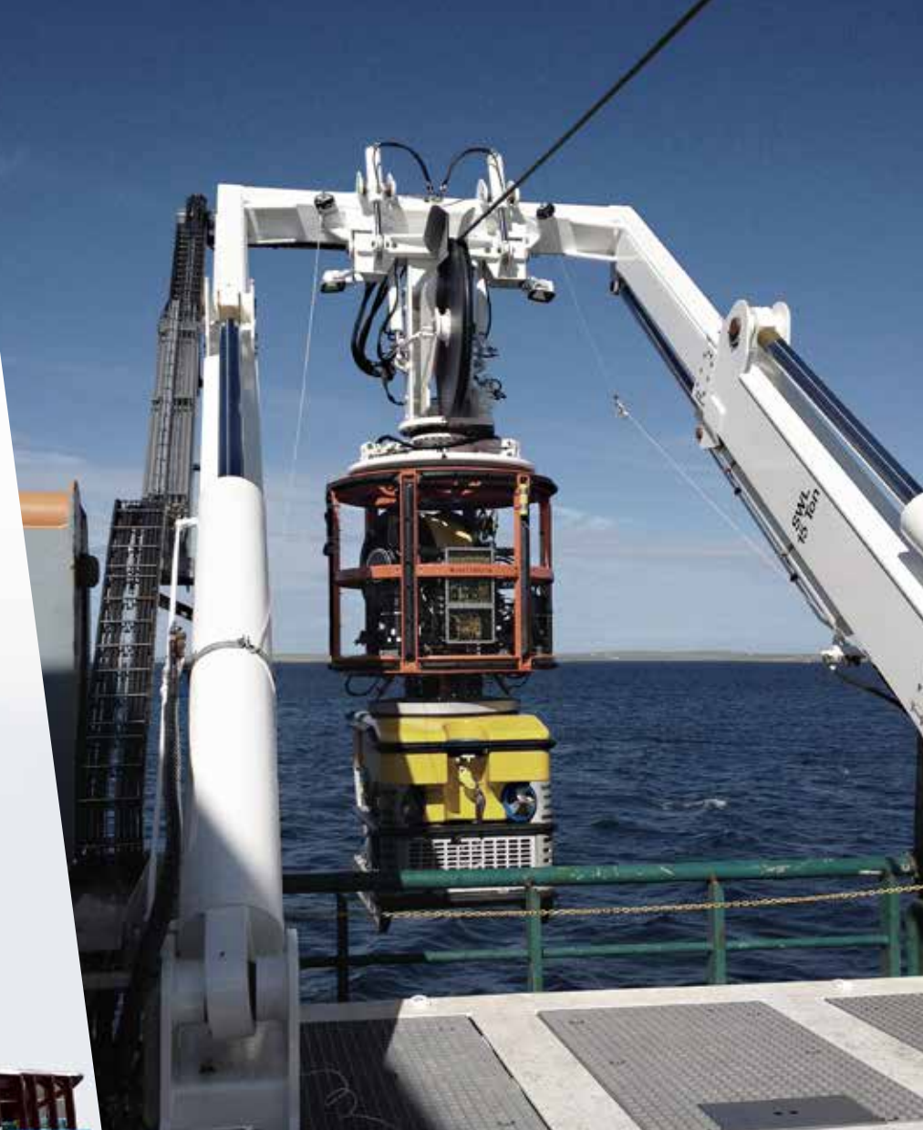
Deck mounted DPL™ - Compact solution for limited deck space. The DPL™ lifts the ROV and TMS between the legs.
