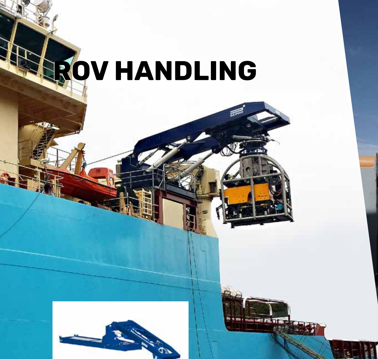
Deck mounted HPL™ - Suitable for limited deck space and narrow hangars. Extensive outreach and excellent dipping functionality.
