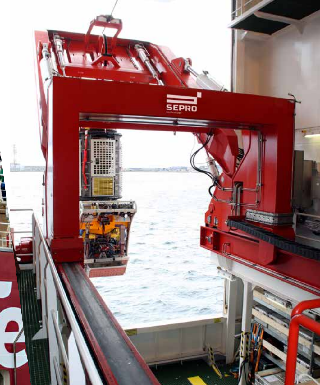
Wall-mounted Rail System WRS™ - Increased lowering capabilities and clean deck area giving space to ROV operation, service and maintenance.
