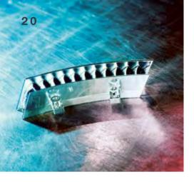
3D printing means the guide vane segments that go into an MAN gas turbine can be printed in a single piece. In the past, they would consist of twelve separate guide vane parts.
