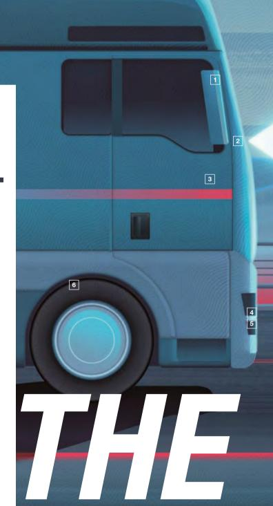
Antennas transmit signals - which is how the vehicles exchange data. The signal is transmitted via ITS-G5, a WiFi standard that was developed for vehicle-to-vehicle communication.
