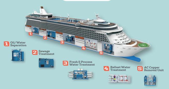
Water and wastewater treatment systems for ships, ports and offshore installations
