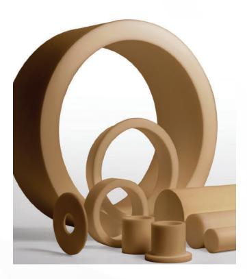
Crossflon® J is gold in colour and has been specifically formulated to operate against soft mating surfaces such as aluminium, brass, mild steel, other plastics and stainless steel. This material possesses no hard or abrasive fillers, has a low coefficient of friction, good creep resistance and compressive strength along with very low wear rates in comparison to unfilled PTFE.
