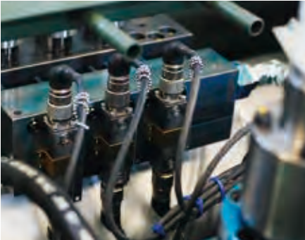
Injection control unit
