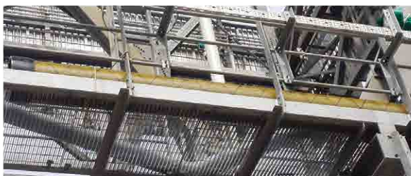
Case 2 Chemical & Asphalt Tanker in AVIC: GRE pipelines system used in Ballast Cargo Area, Cargo Tank gas Freeing, Ventilation and Air Drying, Tank Cleaning
