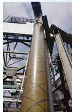
Case 2 Chemical & Asphalt Tanker in AVIC: GRE pipelines system used in Ballast Cargo Area, Cargo Tank gas Freeing, Ventilation and Air Drying, Tank Cleaning
