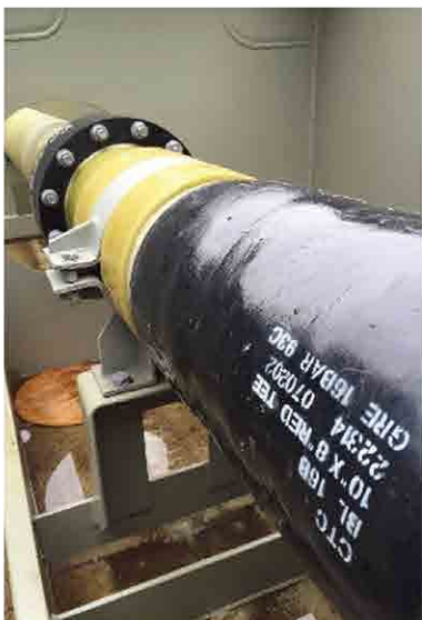
Case 2 Chemical & Asphalt Tanker in AVIC: GRE pipelines system used in Ballast Cargo Area, Cargo Tank gas Freeing, Ventilation and Air Drying, Tank Cleaning
