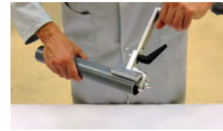
Chamfering the pipe
