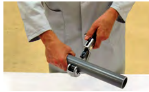
Cutting the pipe to length
