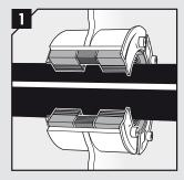
The Roxtec RS PPS/S seals around the thermoplastic pipe against leakage of water and gas through the steel division. Inside the seal, we have added a special fire-stopping material.
