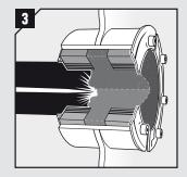
Should a fire occur and the plastic pipe start to burn and melt, the opening will close completely to prevent fire and smoke from spreading through the bulkhead or deck.
