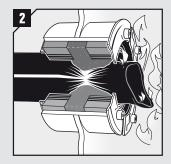
This material will expand and close the middle void of the pipe whenever exposed to high temperatures, such as during a fire.
