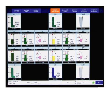
**SUMMARY** SCREENS FOR SERVICE TANK, BALLAST TANK, CARGO PRESSURE, PUMP AND MANIFOLD, CARGO ULLAGE, AND CARGO TEMPERATURE.
