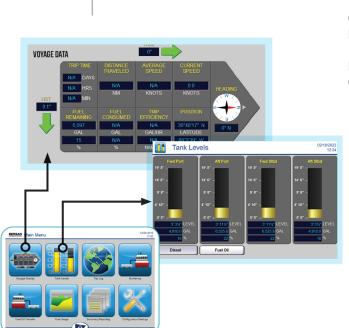
**CONSUMPTION ANALYSIS** WITH GPS COORDINATES FOR ALL INSTRUMENTED BUNKER TANKS.
