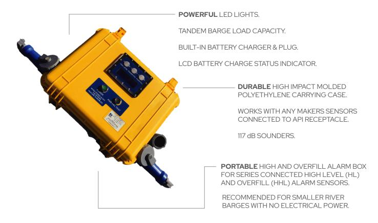
The GUARD LEVEL® Portable Alarm Unit (PAU) is a rugged portable solution for on-board alarm annunciation on inland and coastal river barges. The system monitors and raises alarms through series-connected alarm sensors and gives a unique warning for both High Level (HL) and Overfill Level (HHL) This battery-powered unit plugs into existing tank barge API receptacles. It complies with all CFR regulations for tank overfill control.
