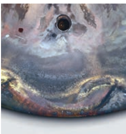
An example of increased crown temperatures leading to severe lacquering on the underside
