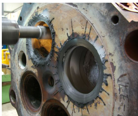
The cylinder cover is machined after welding
