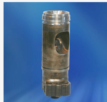
The new valve seat mounted before welding
