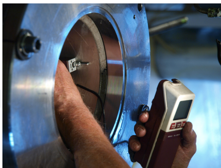
Measuring of surface roughness RA value
