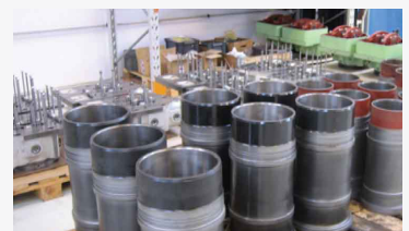
Cylinder liners after cleaning and honing
