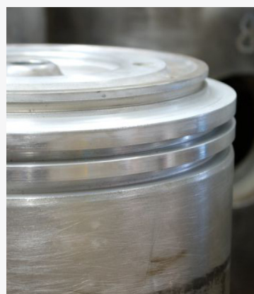
Machined after welding
