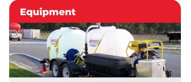
Perimeter Solutions PHOS-CHEK mixing equipment provides easy mixing for support of air tanker, helicopter and ground operations. We also offer equipment for the application of fire retardants, foams and gels. Systems can be fabricated and customized for a particular need.
