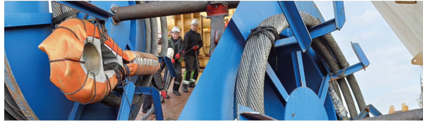
400 tons crane sheaves & ø 72 mm cable replacement, BWTS installation and sheaves restoration. Location: Klaipeda, Lithuania.
