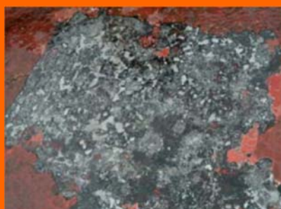
Surface - Rotating Nozzle 500bar
