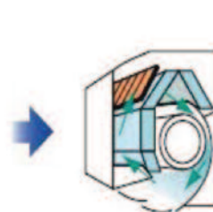
Self clean operation dries the filter and removes moisture
