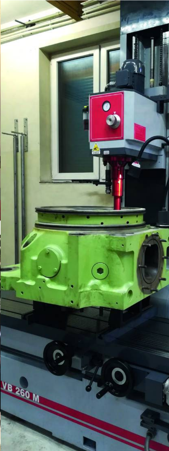
MEDIUM SPEED ENGINES – REBORING OF THE VALVE SEAT RINGS FOR THE OVERSIZE
