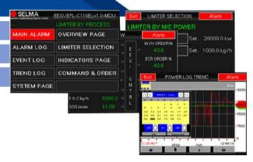
**SELMA SHaPoLi** during adverse weather conditions, this control mode allows for minimizing the wear and fatigue imposed to the Main Engine, the propeller shaft and its components in such adverse and unfavourable conditions. This standard feature, combined also with the vessel **Constant Speed** control mode, make the SELMA SHaPoLi system a complete and robust solution for both fuel oil consumption and speed management, available for the vessel's crew and its operators.
