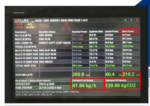
**SELMA SEES** is a unique system based on advanced control techniques in order to improve E/R Power balance and reduce D/G Fuel Consumption. The optimization of vessel's air ventilation and cooling water system involves Variable Frequency Control of the E/R Fans and the Cooling Sea Water Pumps (CSWP/P) according to temperature and pressure feedback signal from the process.
