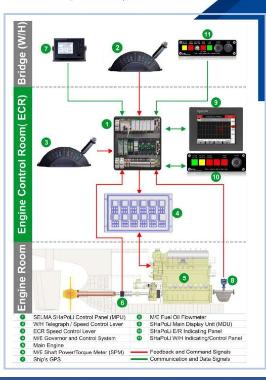
SELMA SHaPoLi monitors in real-time and receives as control feedback the actual power output of the engine through the shaft power meter in relevance with the speed commands. engine's When the power approaches the designated fixed EEXI power limiting setpoint, the SHaPoLi intelligent control automatically takes over and regulates the propulsion command to the engine, accordingly, bypassing control levers and telegraph transmitter in order to limit the power output.
